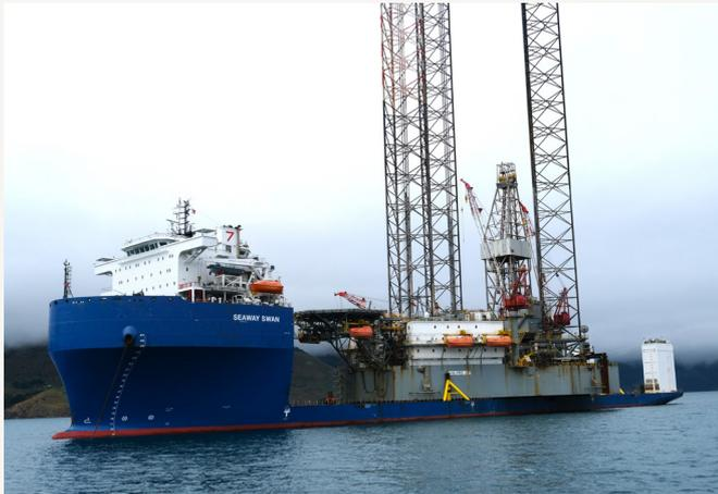
Valaris 107 jack-up rig on heavy lift vessel on route to Kupe Well Head, Taranaki.
